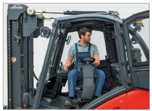
The entire workstation including seat, operating unit, steering wheel and pedals can be adjusted to the desired position with the help of a single handle. With just light movements of the head, the driver always has an optimal view of the driving direction — even during reverse travel.
